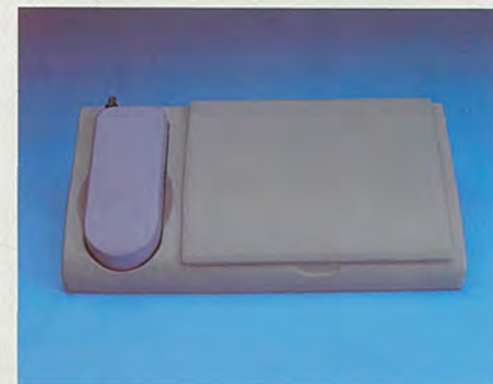
Above: MINT is an integrated cellular fax device that offers the option of a detachable phone. Users can input data via the keyboard, and use the pen to select on-screen menus. Below: Exploded perspective of MINT showing internal details. Bottom Right: AutoCAD is a useful tool to establish the production requirements of parts. Right: The more subdued blue-grey tones relate MINT as a business product.
