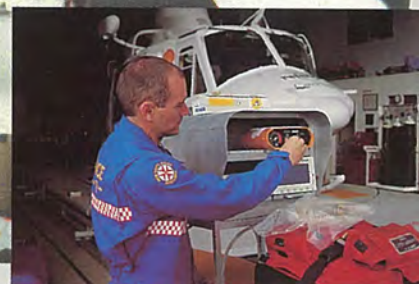
Below right: The unit is placed at the end for structural reasons & for ease of use with obese patients.
