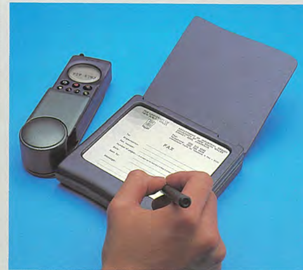
Detachable mobile phone: The GSM phone acts as a wireless modem giving access to the phone line for a variety of data transmissions whilst on the run (phone calls, fax, e-mail). The offer resembles a mini office which fulfils the demands of individuals whom aim to stay in touch, constantly.
