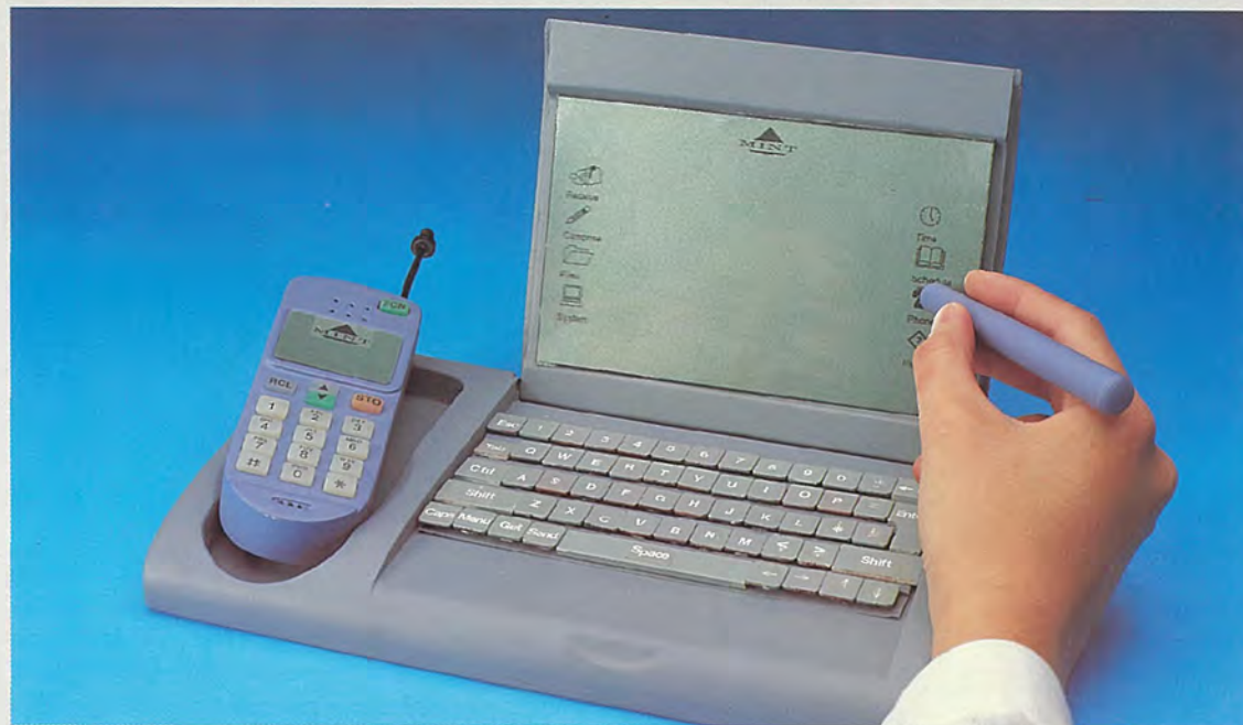
Above: MINT is an integrated cellular fax device that offers the option of a detachable phone. Users can input data via the keyboard, and use the pen to select on-screen menus. Below: Exploded perspective of MINT showing internal details. Bottom Right: AutoCAD is a useful tool to establish the production requirements of parts. Right: The more subdued blue-grey tones relate MINT as a business product.
