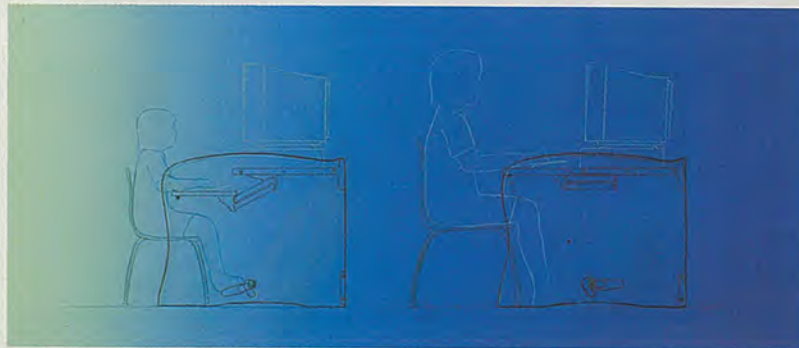
Below: Ergonomic diagram depicting smallest (5 year old) and largest (12 year old) users. PC's may have the monitor placed to the side of the terminal if frequently used by the smaller students. The top height for the keyboard bench is 640mm and the lowest is 520mm. The footrest may be set at a level of zero, 40mm and 100mm.
